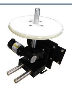
Bottle Separators use a belt or a wheel to put space between containers on a packaging line. Space between bottles may be required for certain packaging functions. For example, to ensure only a single label is applied to each bottle on a conveyor. Separators may also be used to move containers over deadplates connecting conveyors on an automated, turnkey packaging line.
